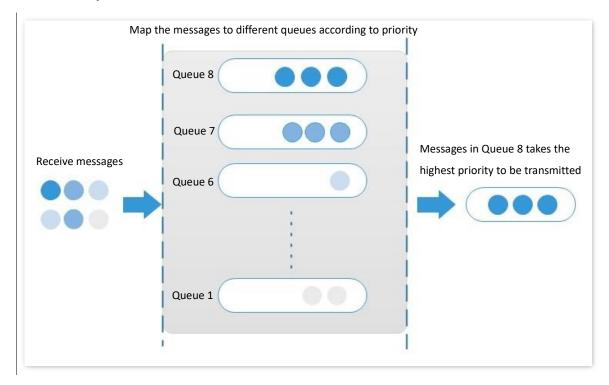
Strict priority scheduling algorithm is specially designed for critical service applications. An important feature of critical services is that they demand preferential service in congestion in order to reduce the response delay.
